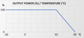
Thus if the charger is forced to operate in an environment above +50°C, it will simply reduce its output power to the corresponding value in the above chart and continue normal operation.
