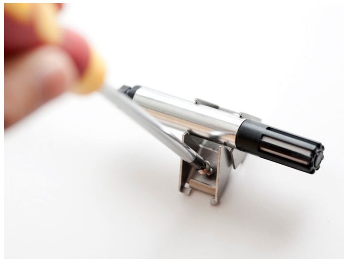
Figure 10 Tightening the Lower Clamp Part
